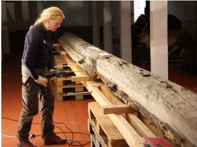
Sample 02960019. Charlotte Kure Brandstrup is taking a core sample from the keel. Photo: National Museum of Denmark
