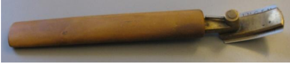
Fig. 12. The razor blade knife, utilized to make a path for measuring, in the wood sample.
