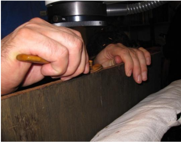
Fig.17. Cutting of the edge of the panel with the razor blade knife under the microscope.
