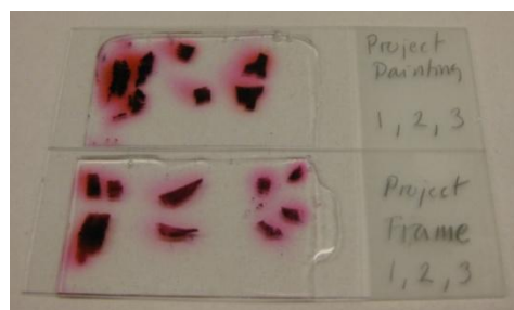
Fig. 11. The samples mounted on a glass slide with Gelvatol and a cover slip. The numbers refers to the different sections as indicated in figure 8 and 9.
