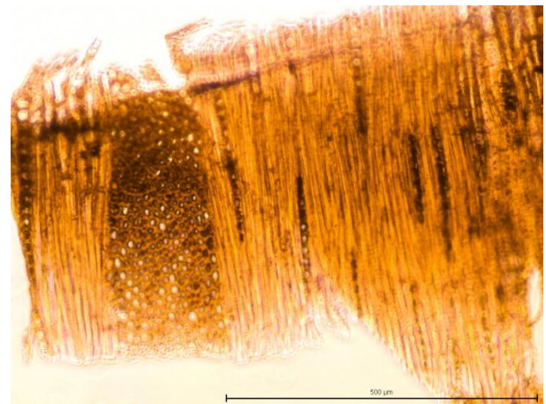
Fig. 20. Tangential section of the panel, with large multi-seriate rays along with smaller uniseriate rays.
