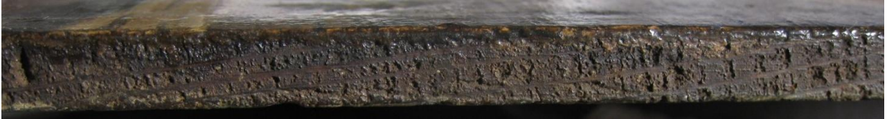
Fig. 14. The proper right edge of the panel which has not been cut. The rays are quite clear, but a precise distinction between the different growth rings is difficult.
