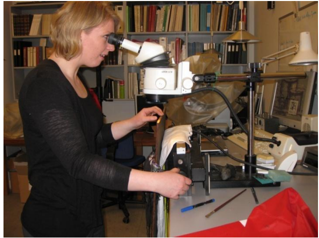
Fig.18. Counting of the growth rings while looking in the microscope
