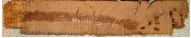
Fig. 13. A path for measuring made with the razor blade knife on a random sample.
