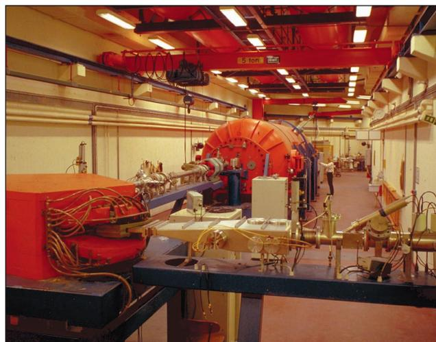
**Fig. 1:** The tandem accelerator at the Institute of Physics and Astronomy, now used mainly for AMS <sup>14</sup>C dating. About 1000 samples are <sup>14</sup>C dated annually. Sample sizes down to as little as 0.1 mg of carbon can be handled.
