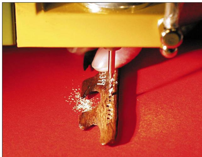
**Fig. 3:** Drilling of a sample for AMS  $^{14}\text{C}$  dating from the tip of a harpoon made of deer antler. Samples of bone are drilled in the same way. Bone collagen is extracted from the sample and combusted into  $\text{CO}_2$  for isotope analysis and dating. Experience shows that collagen preserves the carbon isotopic ratios intact.
