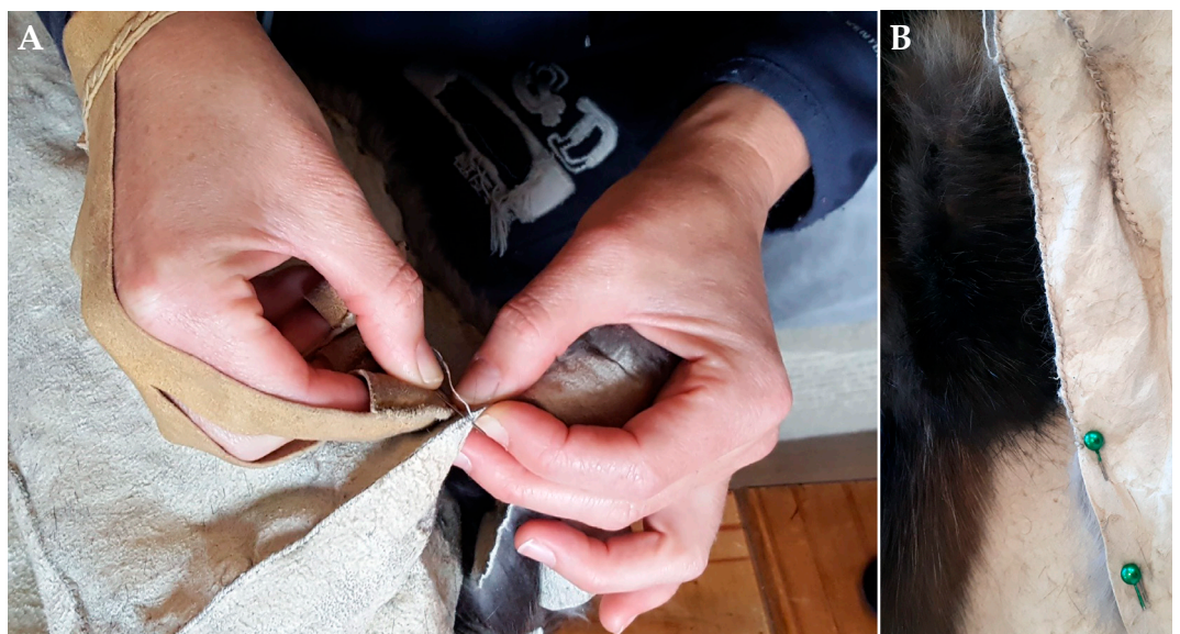
► Fig. 8.11: Sewing using a whip stitch (overcast stitch).
