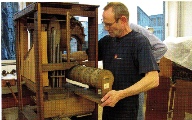
Konserveringstekniker Peter Henrichsen skifter valse. Conservator Peter Henrichsen changing the barrel. Photo: Bodil Holstein.
