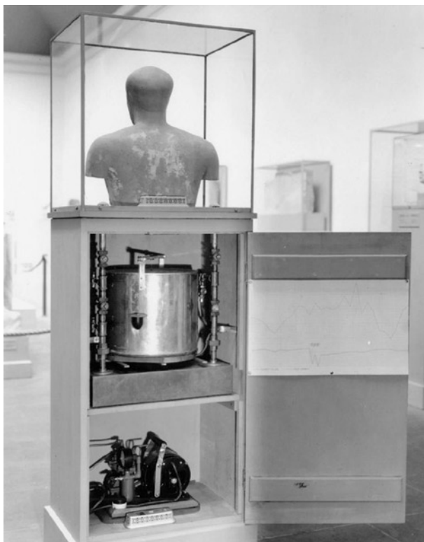
Figure 2. Electrically assisted passive humidity controlled display case, 1938
