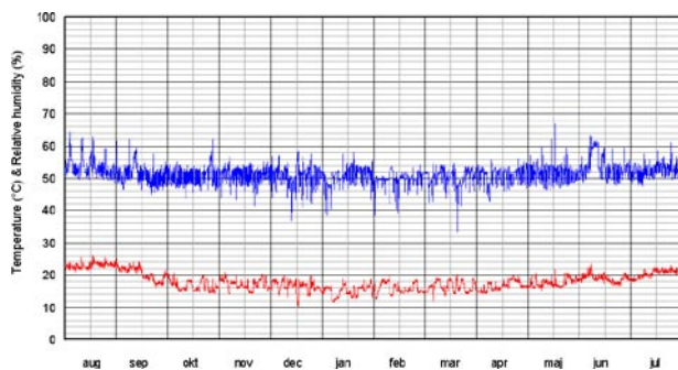
Figure 11. Climate records from Karlslunde church south of Copenhagen. The RH is controlled to 45-55% all year by a mechanical dehumidifier, except for a few episodes, when the RH suddenly jumped to 60% due to a malfunction.
